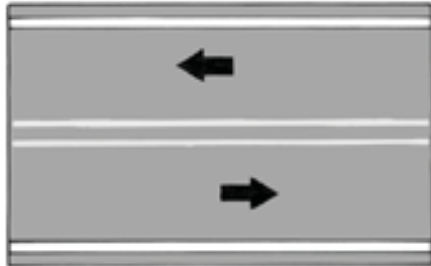
Two-lane, two-way roadway, passing prohibited in both directions, crossing solid lines permitted to turn or in the event of a breakdown.
